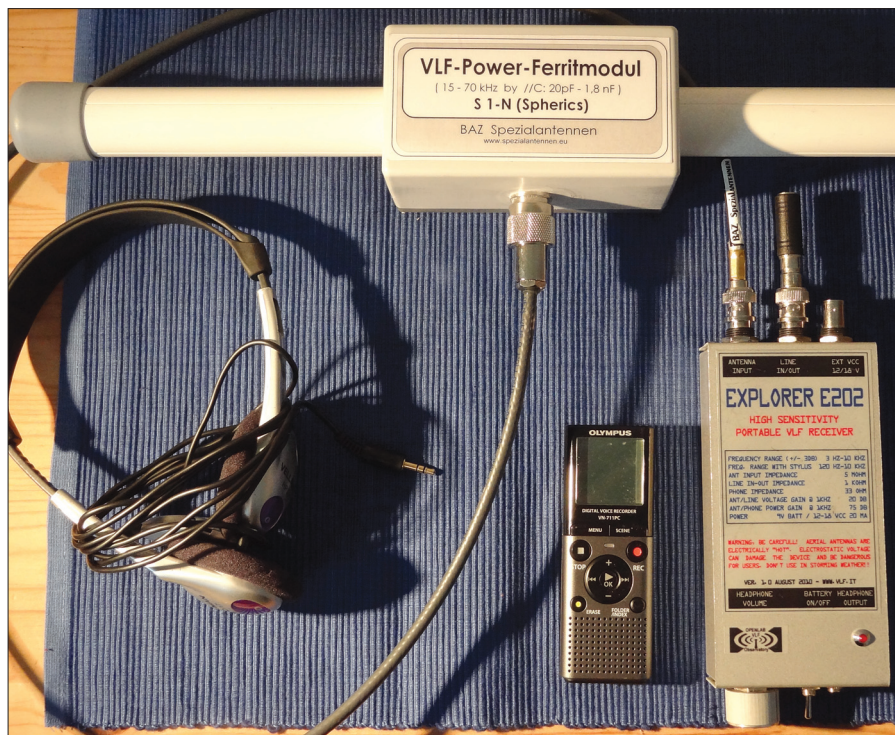
My Explorer E202 receiver, whip antenna, BAZ LFM/S1-N antenna and Olympus digital voice recorder.
